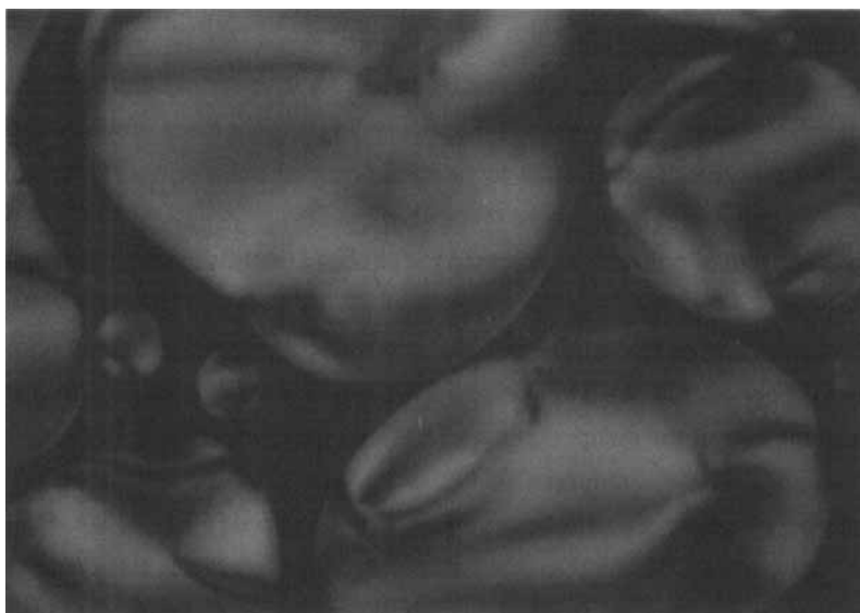
FIGURE 3 Texture of the nematic-isotropic biphasic region in the system composed of 1a /pentadecane at 60 °C, on cooling. (See Color Plate VI).
